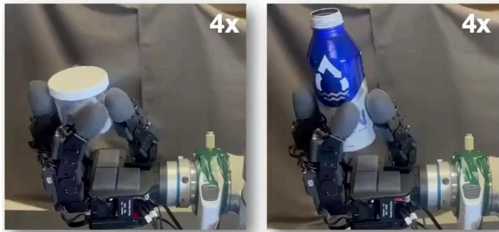
Deployed on touch + proprioception: robust to weight, slip and wrist orientation
