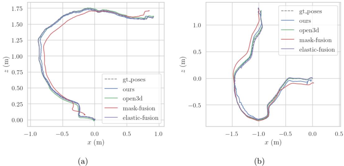
Figure 4.3: Comparison of trajectories between our pipeline and baselines with ground truth. (a) shows *rgbd-scenes-v12* and (b) shows *rgbd-scenes-v14* sequences.
