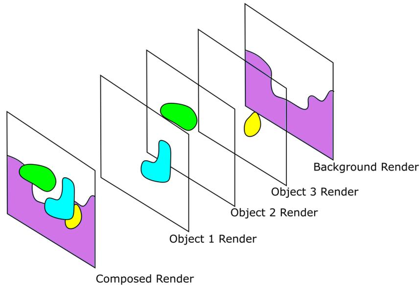
Figure 3.3: An illustration of compositional rendering.
