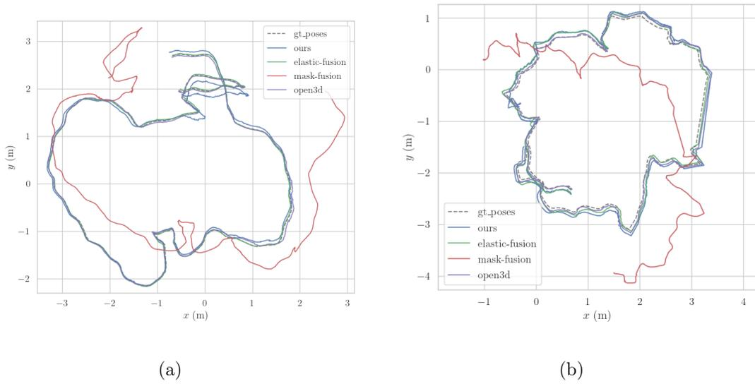
Figure 4.4: Trajectory comparisons on the TUM-RGBD dataset (a) *fr3\_long\_office\_household* and (b) *fr2\_desk* sequences showing that even in the absence of explicit loop closures, our system maintains comparable accuracy.
