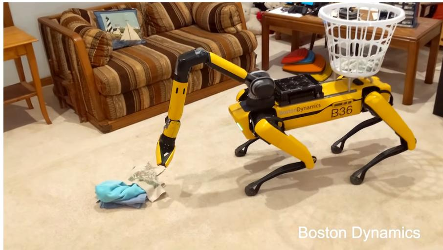
Figure 1.1: Boston Dynamics' Spot Mini robot picking up clothes in a living room. These types of complex interactions require the robot to have a semantic understanding of the objects in its environment.
