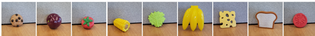
Figure 6: Set of objects for collecting sliding contact trajectories in the Touch-Slide dataset.
